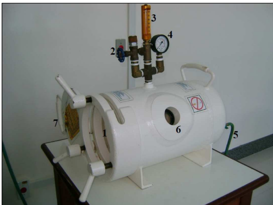
Figure 3 - Hyperbaric chamber with cylinder capsular format built with carbon steel. 1 Entry and exit the chamber; 2 Valve for oxygen escape; 3- thermometer; 4- gauge; 5- tube for oxygen inlet into the chamber; 6- display for observing the animals within the chamber; 7 - Chamber occluding cover. The chamber is 27 cm width, 51cm length and 1.5cm thick.
